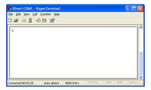
Hit the ENTER key to confirm that the communication with the G-Line unit or T7900 is up and running (A ">" prompt should appear).
