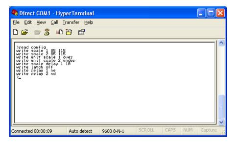
Type the command *read config* or ? at the ">" prompt. The SELCO G-Line relay or T7900 will respond with a list of all valid commands plus its present configuration.
