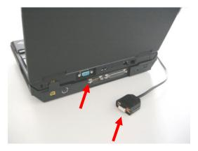
Connect the DB9 female plug of the communication cable to the male DB9 RS232 port of the PC.
