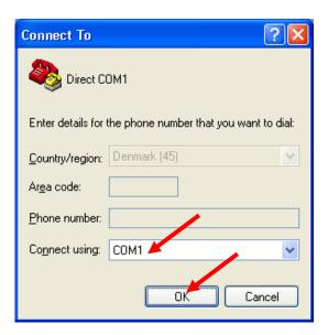
At the *Connect Using* combo box, left click to select the COM-port. Select the COM-port to which the G-Line unit or T7900 has been connected (e.g. *COM1* or *COM2*).
