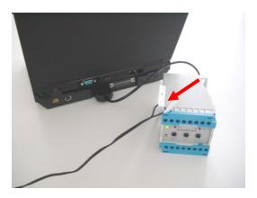
Connect a +24 VDC power supply to the SELCO G-Line relay or T7900. The positive wire (+) connects to terminal 9 and the negative wire (-) connect to terminal 10 of the G-Line relay (terminals 11 and 12 respectively of the T7900). Turn on the power supply and check that the green PWR LED ignites.
