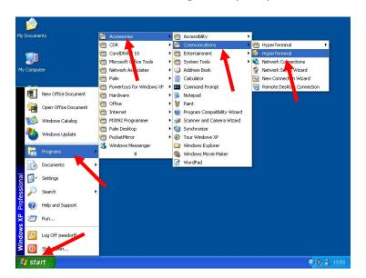
Left click on the *Start* button at the lower left corner to activate the *Windows Start Menu*. Then move the mouse pointer to *Programs*, *Accessories*, *Communications*. To start the application, left click on *HyperTerminal*.
