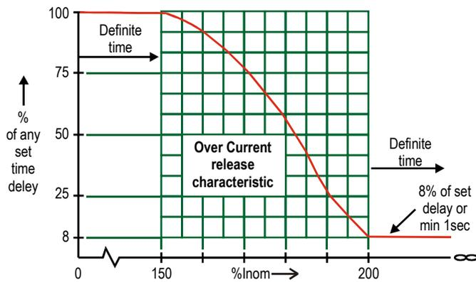
Release characteristic combining definite time and dynamic response to maintain thermal capability protection and selective protection between paralleled generators.
