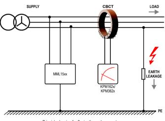
Principle drawing for 3-wire three phase system
