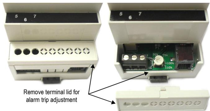
Remove terminal lid for alarm trip adjustment
