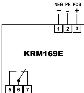
The alarm relay is fail-safe and energises when powered
