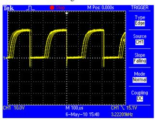
As can be seen on the right hand picture, it is important to trigger the pick-up input from the correct flank. For the NPN pick-up this is the falling flank.
