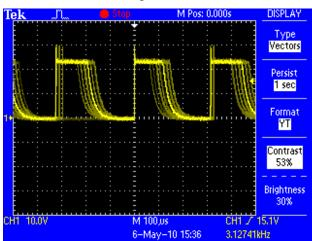
As can be seen on the right hand picture, it is important to trigger the pick-up input from the correct flank. For the PNP pick-up this is the raising flank.
