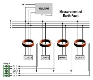
The residual current transformer inputs are split in groups of four channels.
