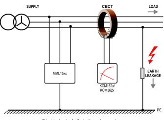
Principle drawing for 3-wire three phase system
